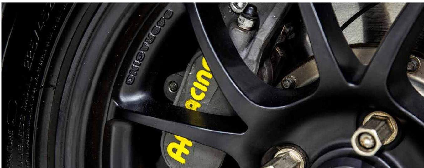
In the case of a power upgrade, he doesn't carry out just a one-off performance test, but a cyclic brake-resistance fade test. This slows the car from 100kph to 0kph several times in immediate succession, ensuring that after repeated applications (simulating a hard twisty and hilly road work-out) you're not going to run out of stoppers.
